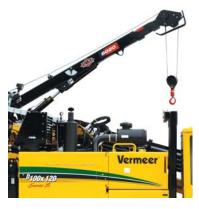
An optional telescopic crane allows the drill operator to change out rod boxes without the use of an excavator or backhoe. The remote-controlled crane gives the operator freedom to move around the drill for improved visibility when replacing rod boxes. The crane has a lift capacity of 7530 lb (3415.6 kg) and a maximum reach of over 20.6' (6.3 m).
