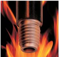
Measured to exact tolerances. Firestick® drill stem from Vermeer is designed to handle high-torque drilling situations while retaining a large inside diameter for superior drilling fluid flow. Constructed of Vermeer specified high-carbon alloy steel, Firestick drill stem features one-piece, forged rods that have been heat-treated for uniform strength and consistent quality.
