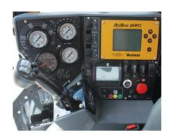
The state-of-the-art operator's station is elevated with an electrically operated swivel-and tilt-control seat. Dual joysticks control functions for drilling fluid flow, breakout vise and throttle, and are integrated into the thrust and rotation controls. This feature provides the operator fingertip control over repetitive drill functions.
