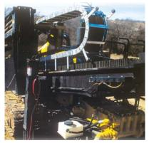
Rack-and-pinion drive. This simple system provides smooth operation. The D100x120 Series II unique narrow rack-and-pinion design helps maintain a small footprint for accessability in congested areas.
